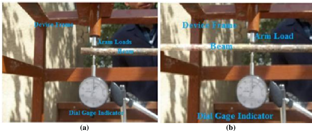
Figure 2: (a, b): Experimental setup cantilever-supported and simply-supported steel beams of deflection measurement by dial Gauge Indicator (DGI) respectively.
