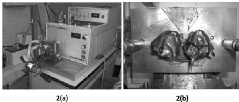
Figure 2: (a) General view Brabender Plasticorder PLE 331 (b) Mixing chambers and rotors at the end of the mixing process
