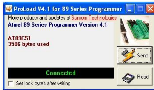
Fig 4.4: Writing the programs bytes onto the microcontroller
